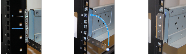
Fig. 17.18: Rail Clamp Latch
