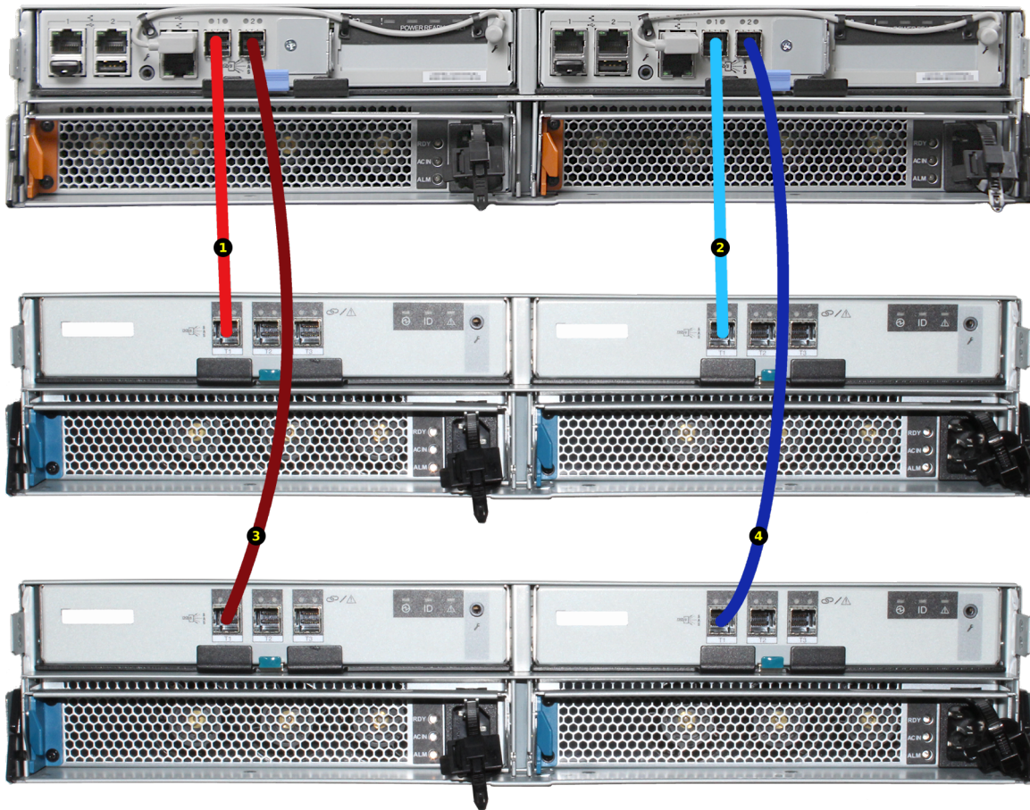
Fig. 17.28: SAS Cable Connection for Two ES12s
