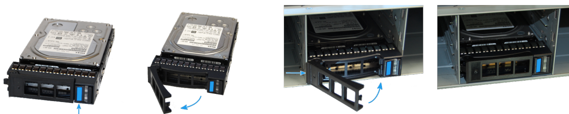
Fig. 16.19: Installing Drive Trays
