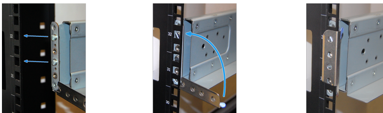
Fig. 16.24: Rail Clamp Latch
