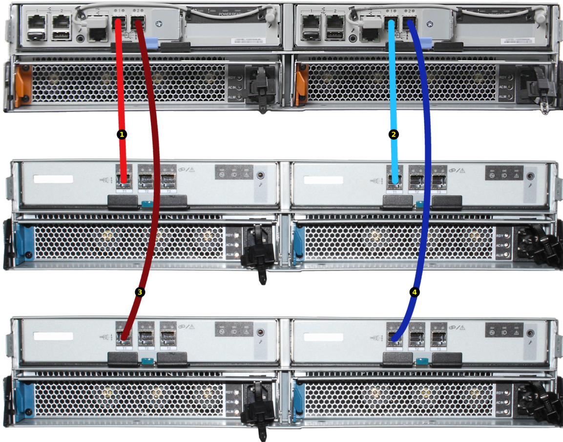
Fig. 16.28: SAS Cable Connection for Two ES12s
